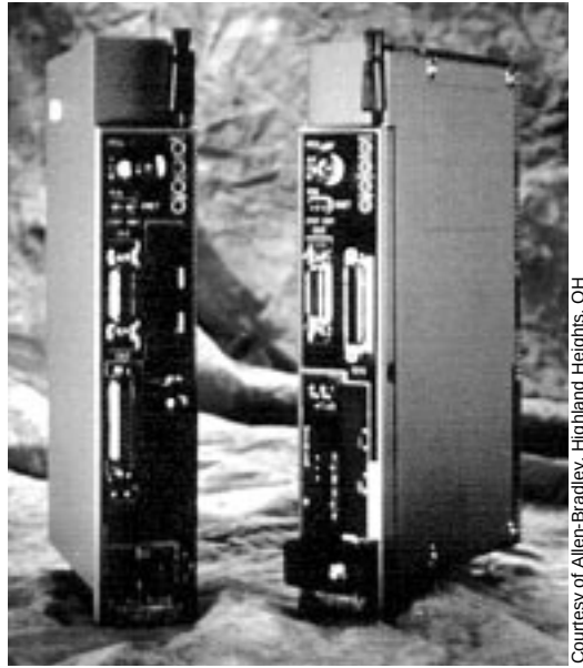
Figure 18-18. Allen-Bradley's PLC-5 controllers with built-in TCP/IP-over-Ethernet protocol.
