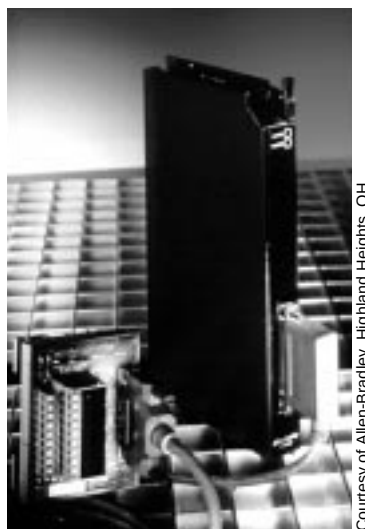
Figure 8-10. Allen-Bradley's Weigh Scale Module (1771-WS).
