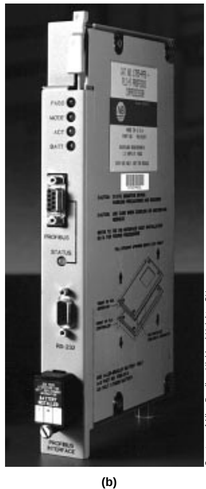
Figure 19-13. (a) Information transfer through a CANbus network and (b) Allen-Bradley's CANbus DeviceNet scanner.
