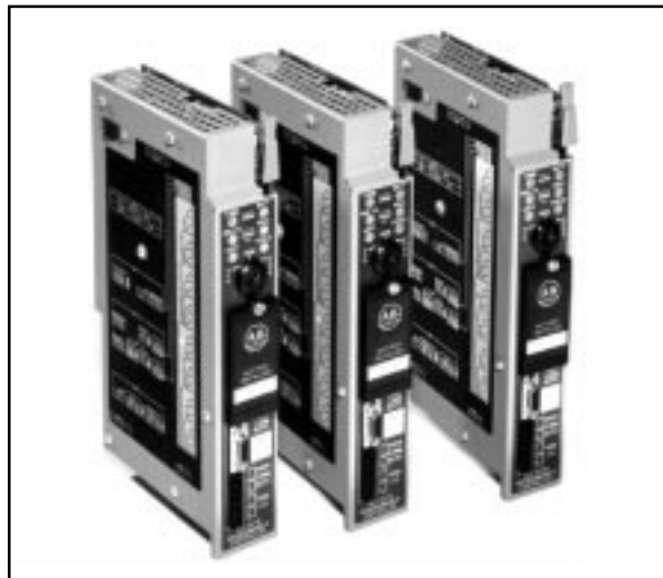
Figure 4-4. Allen Bradley's PLC processors—models 5/12, 5/15, and 5/25.
