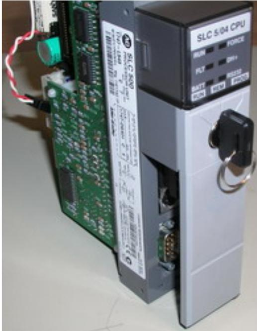
**Run Mode** – is used to execute the user program. Input devices are monitored and output devices are energized accordingly.
