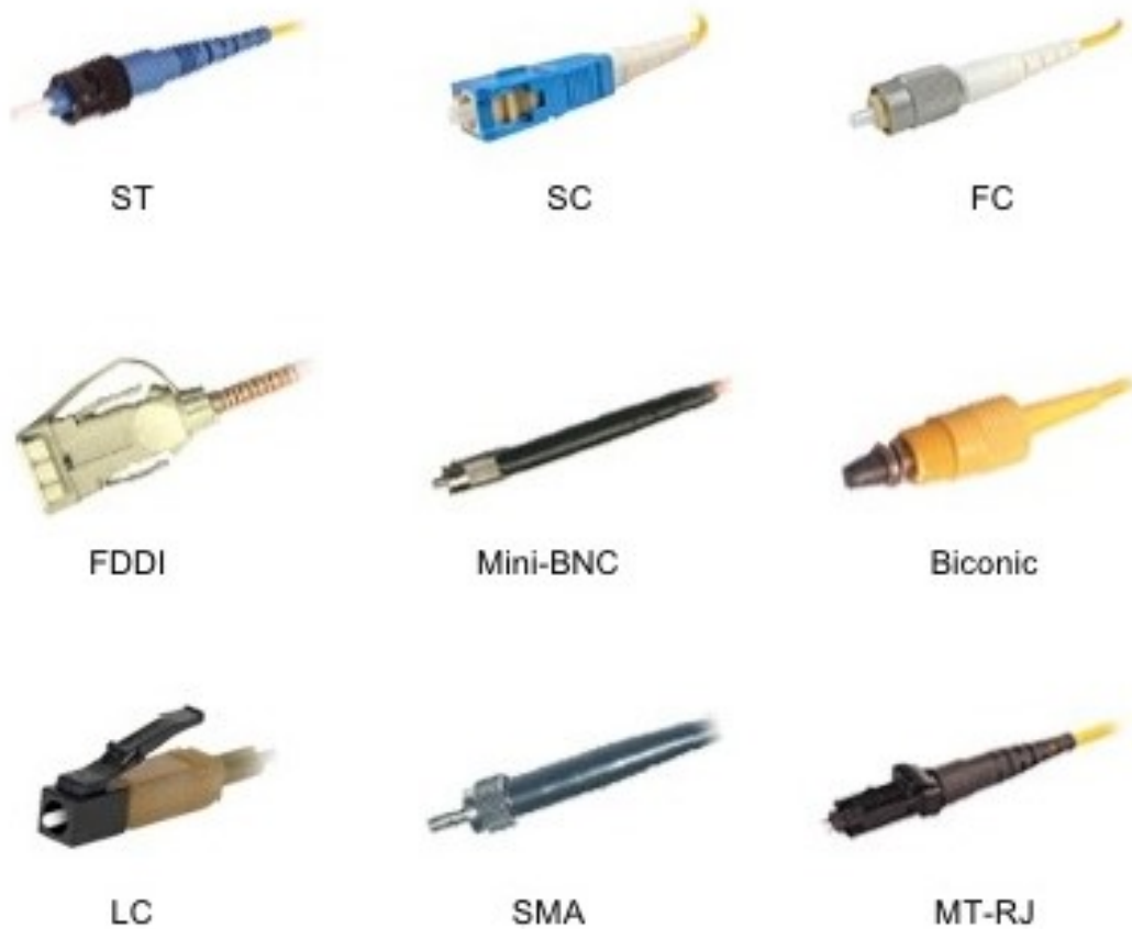
Figure 13: Fiber Optic cable Connectors.
